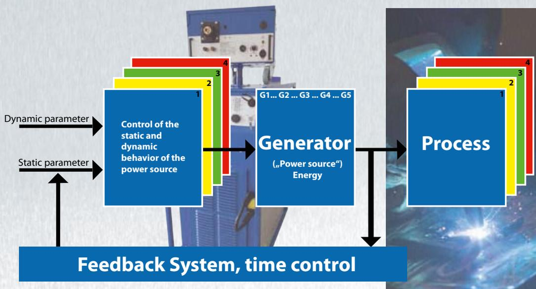
For each different status of the process, a special generator is adjusted, realized by means of a specific static and dynamic behavior of this generator. The parameters required for this purpose are derived from a database in which these parameters have been stored as growing expert knowledge (welding programs).
